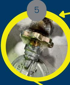
Bubbles Indicate a leak
