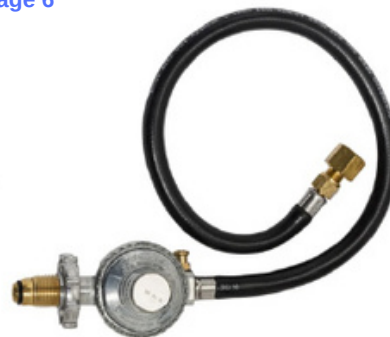
Current type 21 (POL) appliance connection (hose). Phasing out for new LPG appliance by April 2022. Compatible with both New Type 27 (LCC27) and current type 21 (POL) LPG valve
